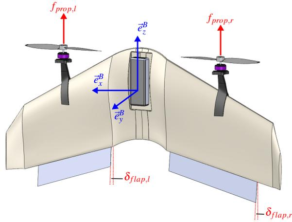
**Fig. 1** Illustration of a flying wing tailsitter vehicle. The vehicle is actuated by two propellers that produce forces along the body  $z$ -axis, and two flaps that produce aerodynamic forces by deflecting the airflow over the wings.
