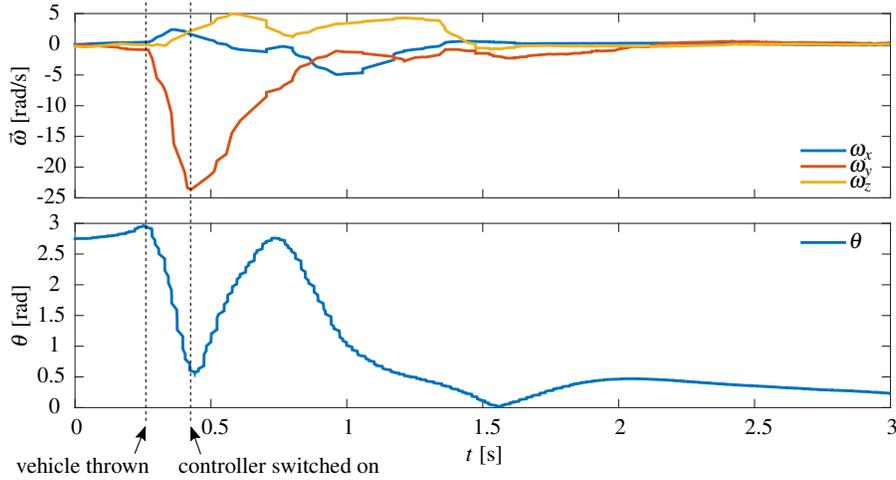
**Fig. 3** Body rate and tilt angle trajectories of an example recovery maneuver. The vehicle is thrown into the air and the controller is switched on at the indicated points in time. Roughly 1 s after the controller has been switched on, the vehicle has recovered to near-hover flight.
