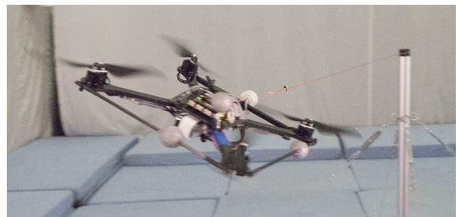
Fig. 1. Quadcopter attached to a tether flying high-speed maneuvers. The tether is attached to a plain bearing mounted on a rigid support structure.
