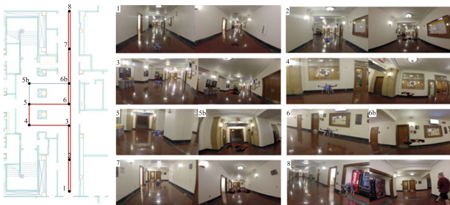
Fig. 7 Long experiment: Blueprint of the experimental area, reference path for the DJI F450 (1-4-5-6-7-8-1) and the Parrot Bebop (1-4-5b-6b-7-8-1), and snapshots of both quadrotors along their paths (1–8)
