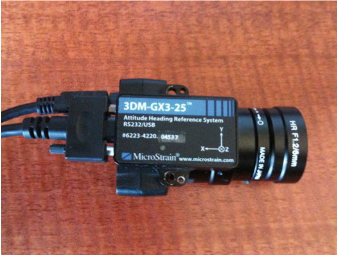
Fig. 1 The sensor suite used in our experiments: A MicroStrain 3DM-GX3-25 IMU is rigidly mounted on a PointGrey Chameleon monocular camera
