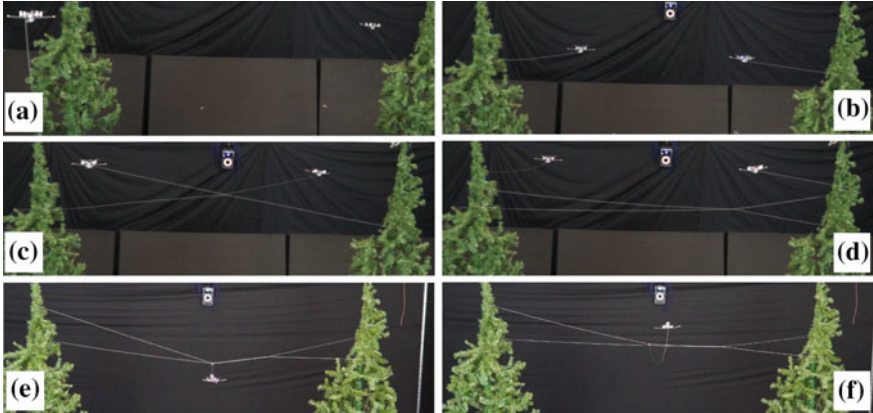
Fig. 7 Two element web construction. Each tensile element is anchored to an environmental feature (a), before winding around the anchor point several times (b) to create a supporting node. Each element is then pulled towards the centre to create a linking node (c), before each drone returns to its original anchor point to secure the web (d). The percher drone then approaches and connects to the web, deactivating all rotors and passively maintaining position (e) before regaining active control and detaching from the web to return to base (f)
