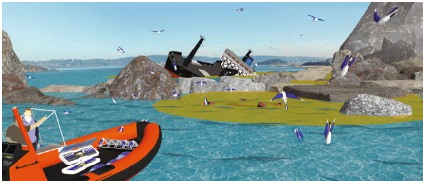
Fig. 1 Plunge diving AquaMAVs map a marine accident, retaking flight in a cluttered aquatic environment using powerful bursts of water jet thrust (adapted from [16])
