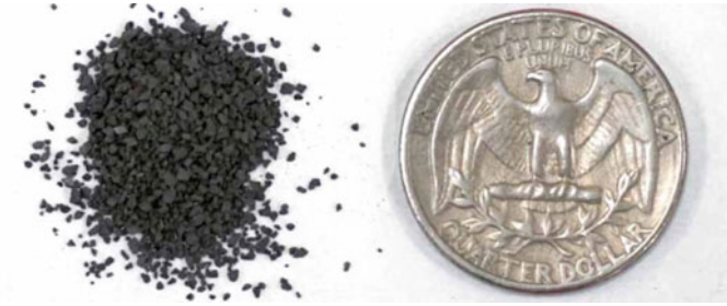
Fig. 3 Calcium Carbide: The 0.5 g of fuel shown here is sufficient for 10 launches of the 34 g thruster presented in this paper
