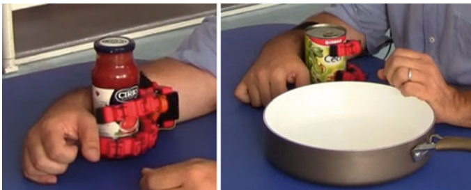
Fig. 10 The Double Sixth Finger as compensatory tool for bimanual tasks. On the left , the paretic hand and the device restrain the motion of a tomato jar so the user can unscrew its cap using the healthy hand. On the right , the device works together with the paretic hand so to let the patient open a can of beans
