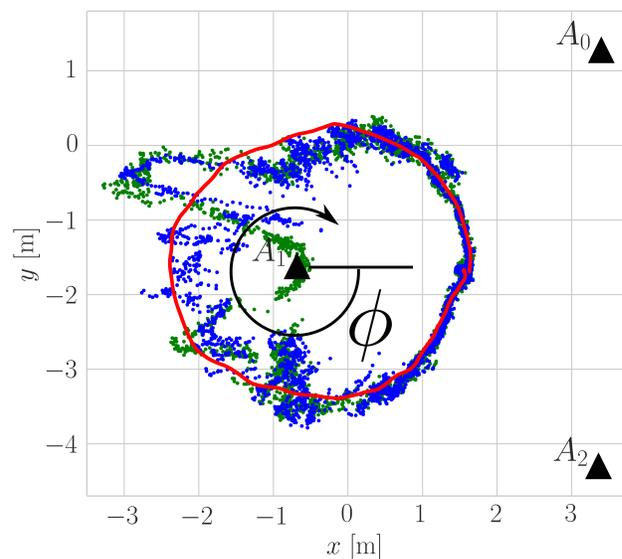
Fig. 5. This figure shows the position estimates generated by an EKF using TOA measurements (blue) and by an EKF using TDOA measurements (green). In both cases, a random-walk model was assumed.
