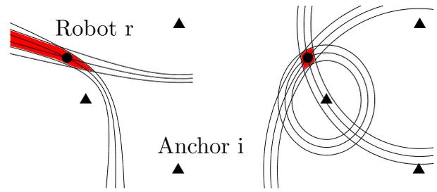
Fig. 2. Geometric solution sets for a given error tolerance. Left: TDOA and TOA localization with unsynchronized clocks. Right: TOA localization with a synchronized clock.
