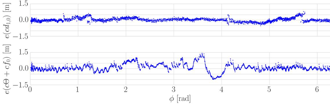
Fig. 6. Upper plot: TDOD measurement error between anchor 0 and anchor 1 ( $e(cd_{1,0})$ ) for the setup shown in Fig. 3 and Fig. 5 for different values of  $\phi$ . Lower plot: Combined error of clock estimate of the TOA EKF described in section IV-C and the TOA measurements of anchor 0 ( $e(c\Theta + cf_0)$ )
