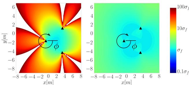
Fig. 3. The variance for an estimator using TDOA or TOA measurements with unknown clock offset (left) and for an estimator using TOA measurements with known clock offset (right). Both plots show  $\sqrt{\text{tr}(\text{Var}(\hat{\mathbf{p}}))}$  for measurement noise with standard deviation  $\sigma_f$ .
