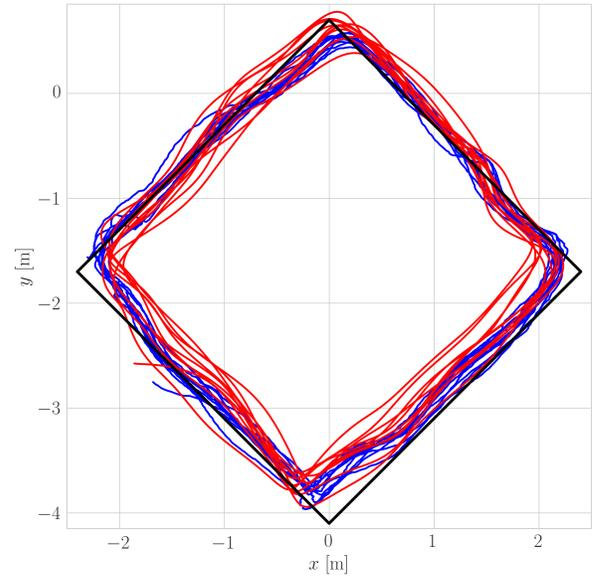
Fig. 7. The position setpoint for the quadcopter was moved with  $1 \text{ m s}^{-1}$  along the reference trajectory (black). The actual (red) and the estimated (blue) position of the quadcopter are shown during this maneuver. See Table I for the anchor coordinates.
