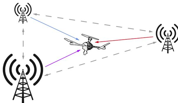
Fig. 1. The architecture of the localization system presented in this paper is shown in this figure. A robot receives UWB radio signals from fixed-position anchors. These anchors periodically transmit UWB signals which are recorded by the robot and used to localize itself relative to the anchors. Since the robot is not active in the communication process, the system allows multiple robots to operate simultaneously and anonymously within the space.
