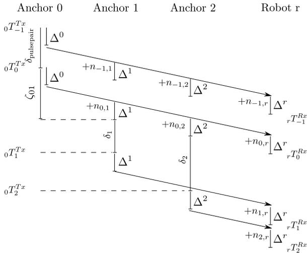
Fig. 4. The one-way communication protocol described in Subsection III-B with the transmission and reception timestamps  $T^{Tx}$ ,  $T^{Rx}$  of the signals
