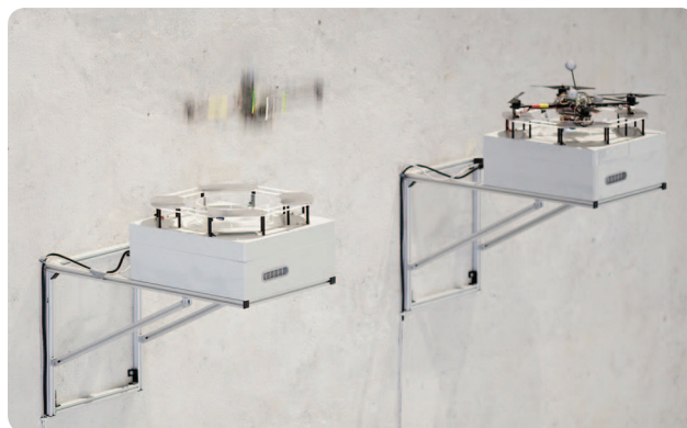
FIGURE 14 Charging stations built to support the continuous operation of the system. The quadcopter’s battery is connected through four charging pads to an off-the-shelf commercial charger and balancer, housed in the lower part of the charging station. (Photograph by François Lauginie.)
