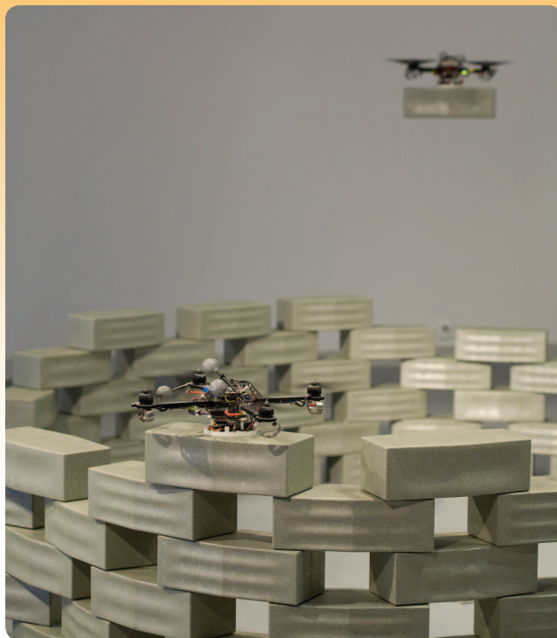
FIGURE 2 Two quadcopters assembling the structure. During the building of the tower, each construction element was required to be at least 1.5 m from the previous element to ensure system safety and to reduce the aerodynamic interference between quadcopters during placement. A construction module is 30-cm long. (Photograph by François Lauginie.)
