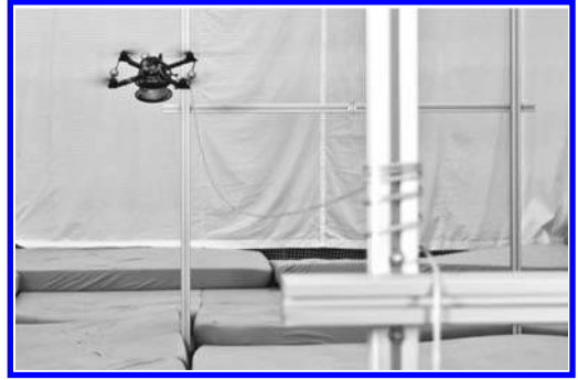
Figure 6. Linear structure. The vehicle autonomously fastens the cable at the existing structure before spanning the link.
