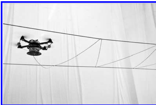
Figure 1. Autonomous erection of a tensile structure by a flying robot.
