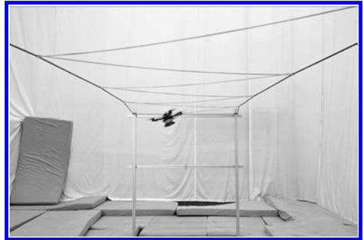
Figure 7. Surface structure. The vehicle constructs a planar structure by flying through and around built components.
