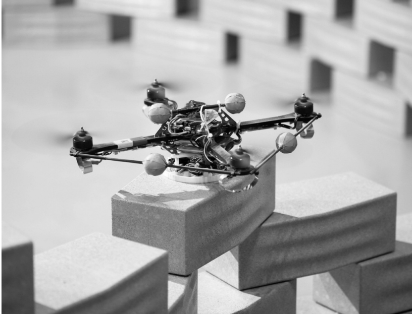
◀ Figure 2: Flight Assembled Architecture: A quadrocopter placing a polystyrene module.
