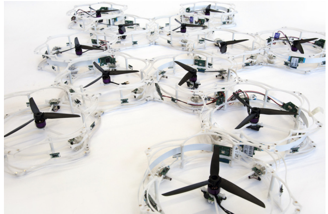
Fig. 1. The Distributed Flight Array is a modular multi-propeller vehicle that can fly in ad-hoc configurations. Configurations may range in size, shape, and sparsity. Designing a controller by hand for every flight-feasible configuration would be impractical.
