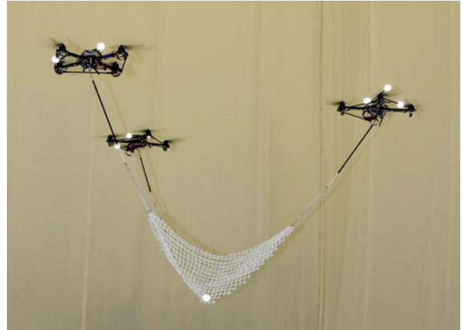
Fig. 1. Three quadcopters attached to a net. Three retro-reflective markers are attached to each vehicle, allowing the system to determine the vehicle pose. The ball, shown lying in the net, is also retro-reflective to be visible to the motion tracking system. The vehicles are placed equally distributed on a circle around the net center.
