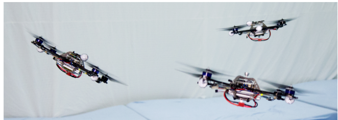
Fig. 1. Multiple quadcopters flying collision-free trajectories in the ETH Flying Machine Arena.
