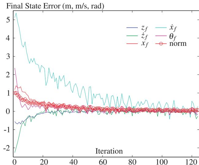
Fig. 11. Final state error and parameter evolution over 124 iterations for a vehicle with  $\theta_{max} = 1300^\circ/s$  using  $\mathbf{J}$  and  $\mathbf{P}^0$  calculated for  $\theta_{max} = 1600^\circ/s$ . Step size  $\gamma = 0.07$ . Note that  $\theta_f$  is normalized to  $(-\pi, \pi)$ .
