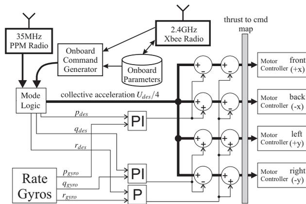
Fig. 7. Logical layout of the onboard controller. The variables  $p$ ,  $q$ , and  $r$  refer to roll, pitch, and yaw body rates, respectively. In the case of the flip maneuver as described above,  $q_{des} = \dot{\theta}_{des}$ , while  $p_{des} = r_{des} = 0$ .
