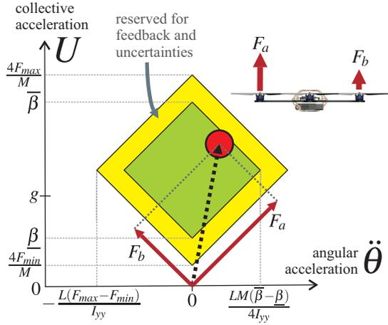
Fig. 4. Control envelope for a quadcopter moving in a vertical plane.
