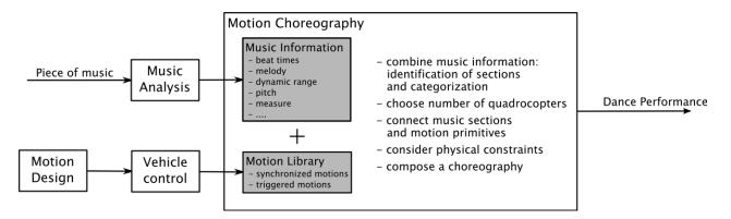
Fig. 7. The proposed platform: combining music and quadrocopter motion into a multi-vehicle dance performance.
