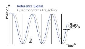
Fig. 4. Reference trajectory in lateral direction (dashed line) with corresponding quadrocopter motion (solid line). Vertical lines represent beat times.
