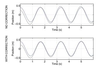
Fig. 5. Quadrocopter response to the dashed-lined input signal for the case of no phase correction (top) and phase error compensation (bottom). The solid line represents the vehicle trajectory.
