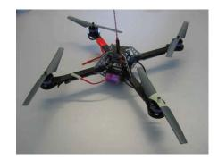
Fig. 2. The quadrocopter, measuring 53 cm in diameter.
