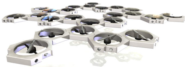
Fig. 1. Shown in this figure is a concept representation of the DFA in a random configuration. The array is composed of interconnected rotor modules that communicate with one another for coordinated flight.
